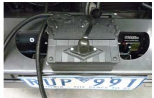
5. Connect three colour coded cables to the corresponding poles on winch motor.
