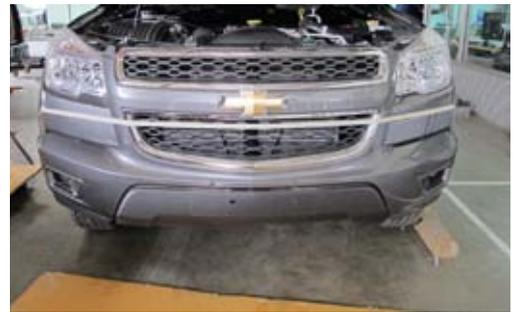
3. Cut along line marked in previous step to remove lower section of bumper bar.
