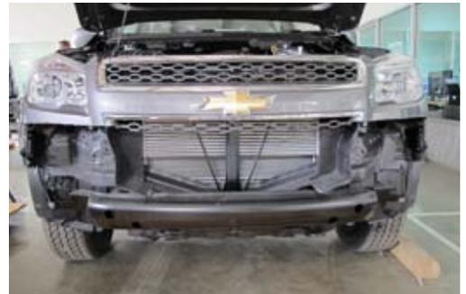
4. Remove bumper bar reinforcement.
