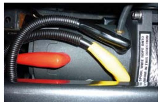
12. Connect the thin black earth wire and negative battery cable to the earth connection on the opposite side of winch motor.
