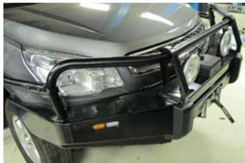
11. Align bull bar with vehicle leaving a 10mm gap between bullbar wing and mudguard. Tighten all bolts.
