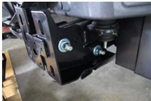
7. Using chassis bracket as a guide, drill a 12.5mm hole through chassis and install bolts, flatwashers, spring washers and nuts as shown,
