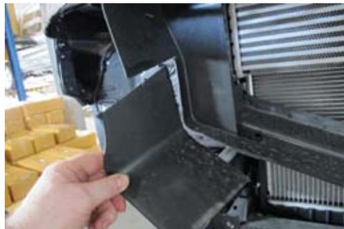
6. Install chassis brackets as shown using hardware provided.
