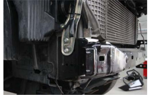
3. Remove bumper support frame. This is also held in place by sealant so many need leverage to assist removal. Place supplied chassis strengthening bracket to bumper support frame as shown.
