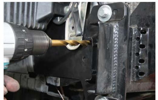
10. Drill 10mm hole into frame as pictured. Only drill through the outer wall of chassis.
