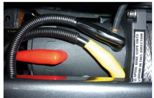
5. Connect the thin black earth wire and negative battery cable to the earth connection on the opposite side of winch motor.
