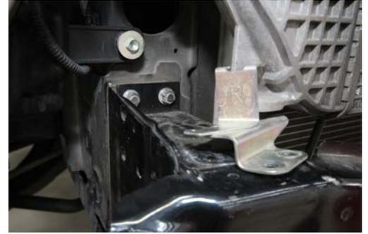
7. If winch is being installed, it needs to be attached to mounting cradle before cradle is attached to the vehicle.
