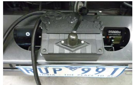
4. Connect three colour coded cables to the corresponding poles on winch motor.
