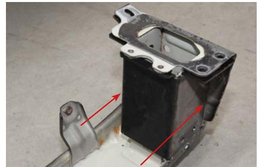
4. Drill out spot welds with 6mm drill.
