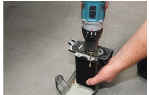
5. Bolt support to frame with M6 bolts and nuts supplied.
