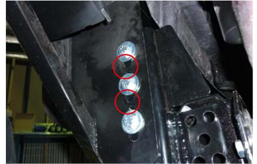
17. Fit protection plates underneath the bull bar using M8 bolts, spring washers and flat washers provided.
