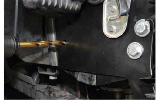
11. Open up access hole under frame as pictured to allow installation of nuts.
