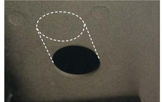
12. Fit wired nut and bolt set supplied through hole just created.
