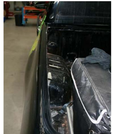
5. Using supplied neutral cure silicone seal any seams or holes that might allow water to enter the tub once canopy is installed.
