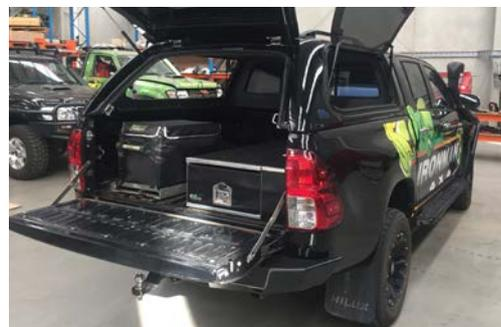
8. Close the vehicle tailgate and adjust the position of the canopy until the rear door closes easily and makes even contact with the tailgate.
