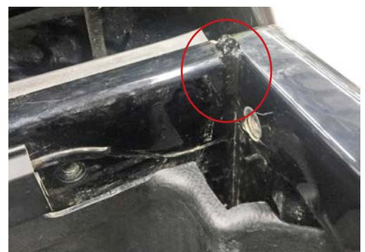
6. Attach adhesive seal to the top of tub and seal all joints with neutral cure silicone.
