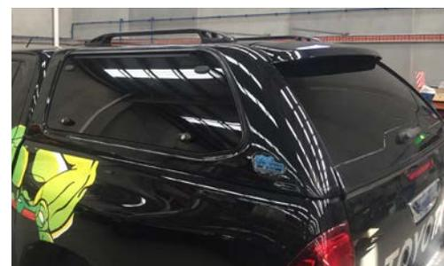
9. Recheck that the canopy is square and aligned evenly with the vehicle tub. Adjust if required.
