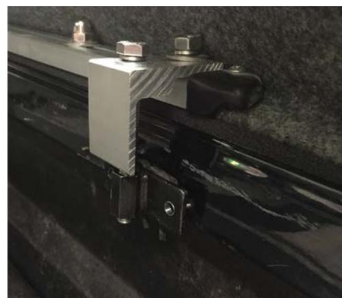
11. Recheck canopy alignment and rear door for ease of opening and closing and adjust if required.
