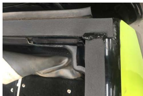
7. Place canopy in position on the tub of the vehicle, being careful not to dislodge the seal.
