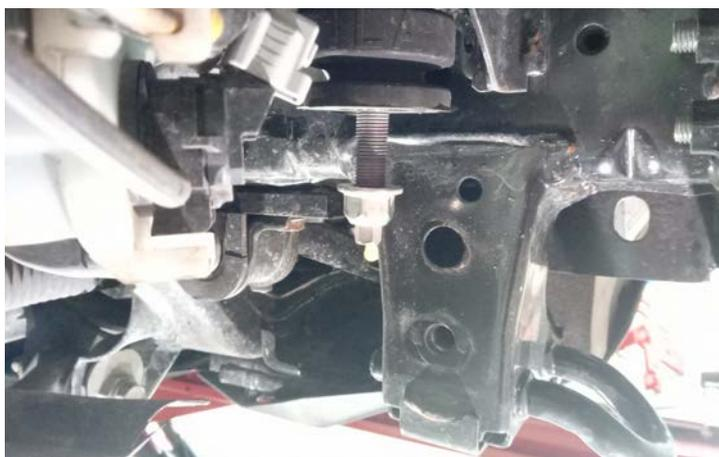
5. Insert the crush tube into the cross member. This may require a slight tap in.
