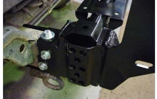
5. Refit recovery hooks using original bolts.
