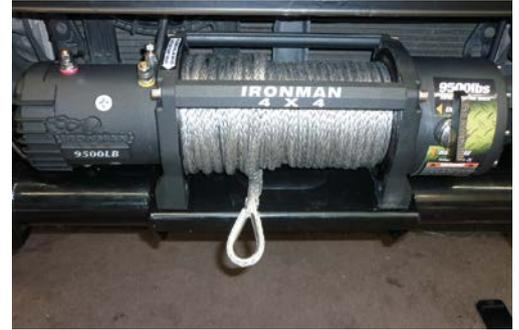
2. Bolt fairlead to recess in front of bull bar using bolts, washers and nuts provided.
