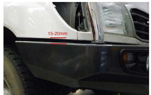
11. Once bar is aligned with vehicle and tightened, drill through pinning holes between bull bar and chassis brackets. Secure with hardware provided.
