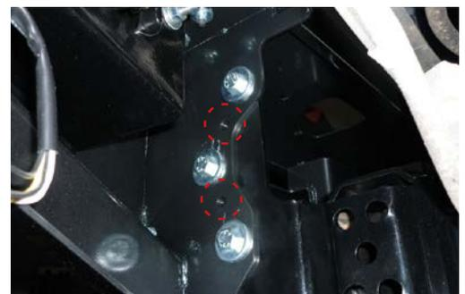
12. Fit protection plate to underneath of bull bar using M8 bolts, spring washers and flat washers provided.
