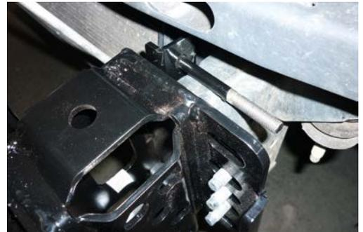
8. Fit chassis bracket to chassis and secure loosely
