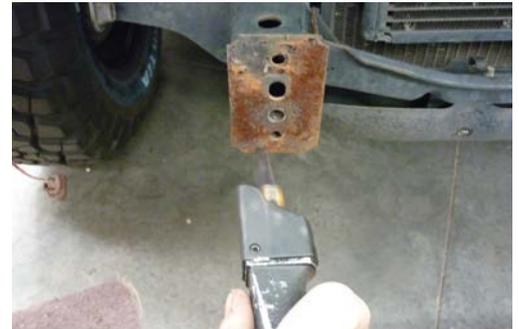
3. Fit chassis bracket to chassis using M10 bolts, flat washers and spring washers into original bumper bolt holes. Refit original recovery hook on right hand side and tie down point on left hand side using original bolts.
